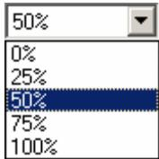
The trigger position defines the amount of information stored in the trace buffer before and after a defined event called the trigger. Once a trigger is encountered a trigger position of 0% stores all events starting at the beginning of the trace buffer.
