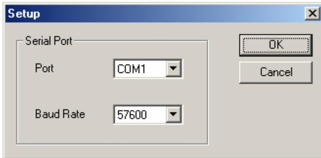
For the RS232 interface, enter the COM port number and the baud rate you are using. The board rate of the analyzer will be automatically adjusted to match the software setting. Select USB if using the USB port.
