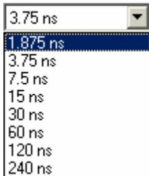
The power zoom sample clock specifies the sample rate of the high speed trace buffer. This buffer samples bus signals around the trigger point and is displayed by clicking on the power zoom button in the state or waveform display.
