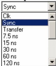
The analyzer samples the bus using either the bus clock or a high precision analyzer clock.
