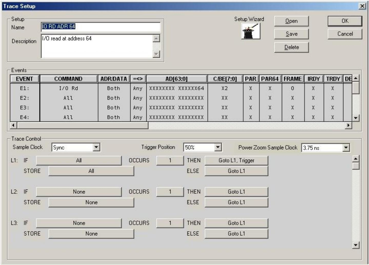
The setup window is divided into 3 main sections: Setup Utilities, Events, and Trace Control.
