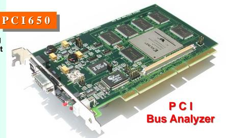
The PCI650 Analyzer operates in 32 and 64 bit systems running from 0 to 66 Mhz. Over 100 protocol and timing violations are automatically checked and correlated with captured bus activity. System performance measurements include Bus Utilization, Transfer Rates, Latency, and Statistics.
