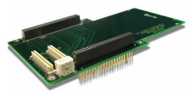
The PMC-to-PC/104-Plus Adapter accommodates one PMC 650 Bus Analyzer Card to a PC/104-Plus environment for PCI analysis. The adapter is stackable and can be used with multiple devices. Additional circuitry allows the adapter to be configured as device 0-4.
